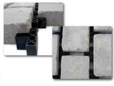
As shown on the pictures above, the PaveDrain® is placed between the paving stones, creating a gap for the drainage of the area. In the following photos this gap is loaded with granite chippings however the space can also be filled with sand, gravel, pebbles or reinforced with grass, where surface water can drain through. Get more information on 86 37 71 33.
